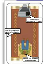
In a home TV installation the loop can be under the carpet, the baseboard. in the basement or in the attic to transmit sound to the telecoils in your hearing aids.
